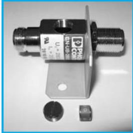
The 7205 has a threaded cap on the side that contains a recess that positions the gas arrester tube in the center of the access hole. The gas discharge tube can be replaced in the event that a lightning strike causes a failure.
